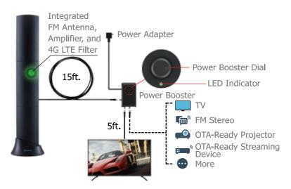
In order to adjust the amplifier gain, use the power booster dial:
