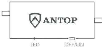
The **Power Inserter** must be powered in order to function. Push the smart switch On or Off and select the switching with which more channels are received.
